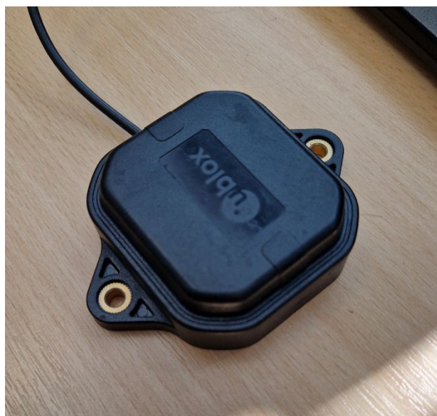
Figure 26. Magnetically mounted GNSS antenna
